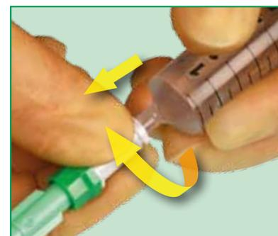
When using a luer-slip fitting, e.g. a non-locking syringe, you will find that a quarter turn of the syringe as it is pushed firmly in will help provide a secure fit.
